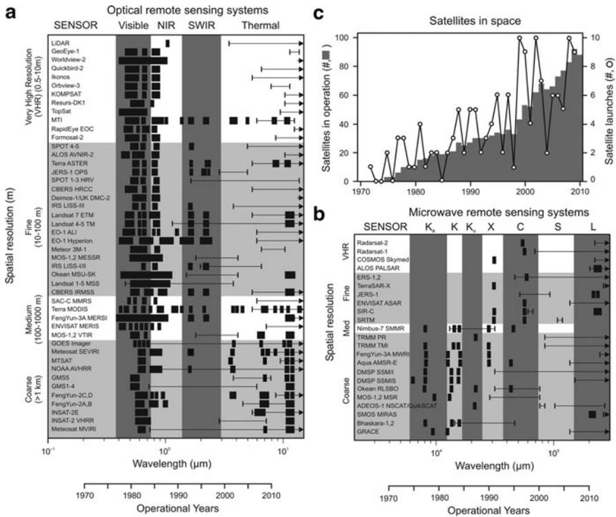
**Fig. 3.2** Remote sensors useful for the study of forest hydrology. For each remote sensor, the portions of the electromagnetic spectrum detected (*black bars*) and the period of operation (line, with *arrow* indicating currently operational) are shown for (a) optical and (b) microwave sensors. The total number of satellites launched (*open circle*) and satellites operating in a given year (*bar*) are shown in (c)
