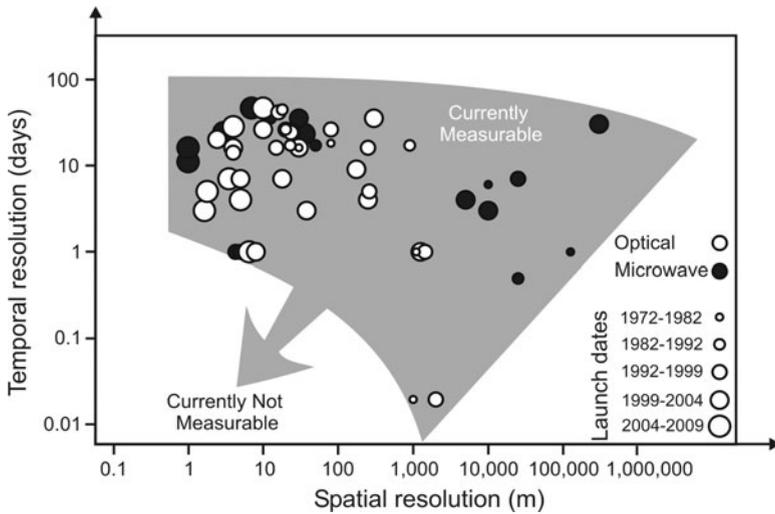
**Fig. 3.3** Spatial and temporal resolution of remotely sensed data with a shaded polygon defining limits of currently measurable resolutions. The *arrow* depicts the additional resolutions needed for many forest hydrology applications
