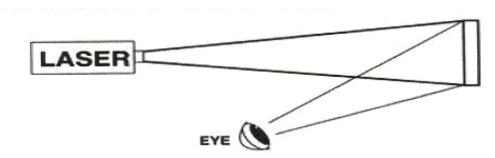
Figure 7 - Extended source viewing of a normally diffuse reflection. Diffuse reflections are not normally hazardous, except with very high power Class 4 lasers.
