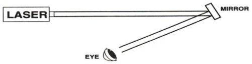
Figure 5 - Intrabeam viewing of a specularly reflected (secondary) beam from a flat surface reflector. Specular reflections are most hazardous when the reflecting surface is flat.
