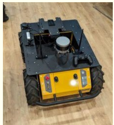
This ground robot is equipped with sensors that capture real-time information about the environment
